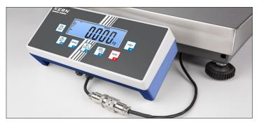
■ Verification plug, for verified balances this enables you to separate the display device and platform without affecting the verification, e.g. for installing the scale in a packing and dispatch table, pit frame etc. at a later date. Please order this at the same time as you purchase your scale, see accessories
