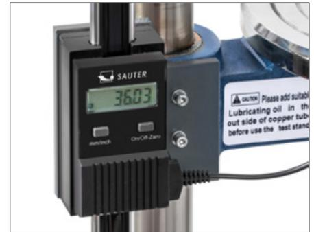
Distance measurement directly in machines or sites with RS-232 interface
