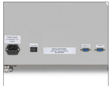
Interface for data transmission from the SAUTER FH measuring device and for controlling the test stand with SAUTER AFH software
