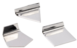
Milligram weights, flat polygonal sheet
