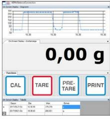
Modern digital weighing transmitter for the rapid recording of weighing data and forwarding it to the most varied output channels such as tablets, networks, SPS controllers, etc.
