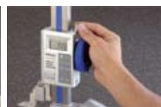
Slider clamping lever
