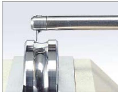
Inner/outer ring contour of a bearing
