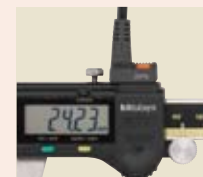
ABS Digimatic Caliper CD-15CX No.02AZD790C
