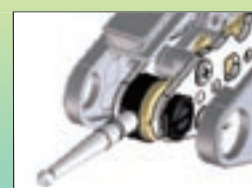
Stylus bearing screw held in sub-plate.
