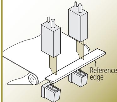
Measurement of spacing of IC chip leads
