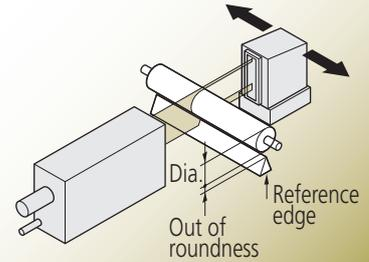
X- and Y-axis measurement of electric cables and fibers
