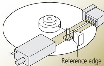
Measurement of gap between rollers
