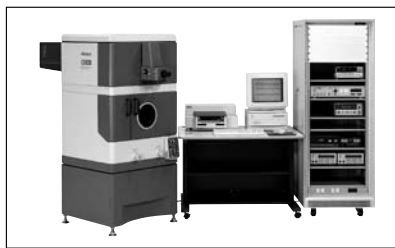
Interferometer used for calibrating gauge blocks (Miyazaki Plant)
