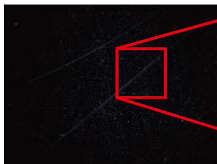
Dark-field: Allows highlighted observation of microscopic abnormalities such as flaws and contamination by using diffused light.
