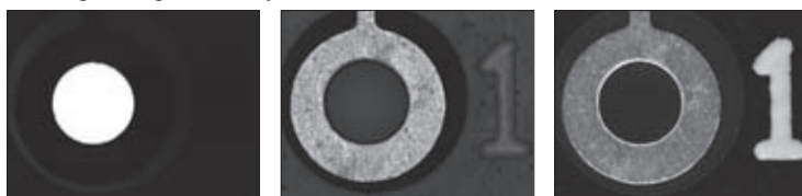
Contour illumination Vertical surface illumination Programmable ring light illumination
