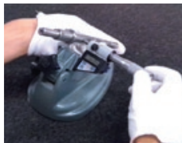
Diameter measurement using a micrometer cannot detect an odd-number lobing condition and resolution is marginal.
