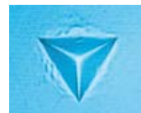
Indentation by triangular pyramid indenter
