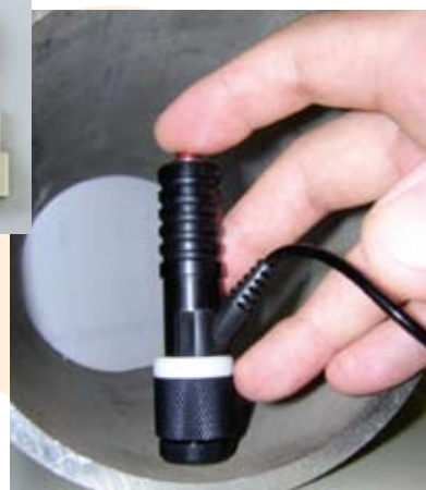
● Hardness testing of internal walls of pipes and tight spaces
