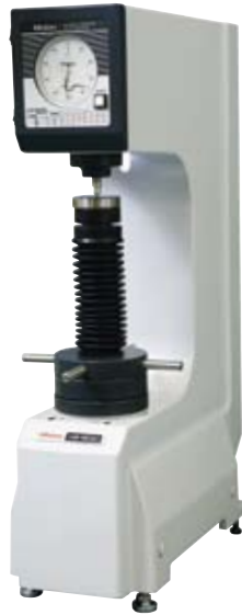
HR-210MR 963-220 Rockwell hardness testing machine
