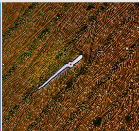
Laser-crystallized silicon on glass, EC EPIPLAN 10x/0.3
