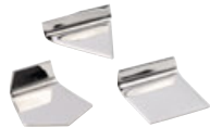
Milligram weights, flat polygonal sheet
