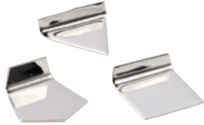
Milligram weights, flat polygonal sheet
