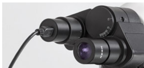
Eyepiece camera fixed into the tube
