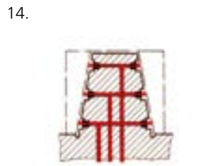
14. Taper pitch measurement as well as form and diameter measurement of an inside taper with taper jet air plug gage.
